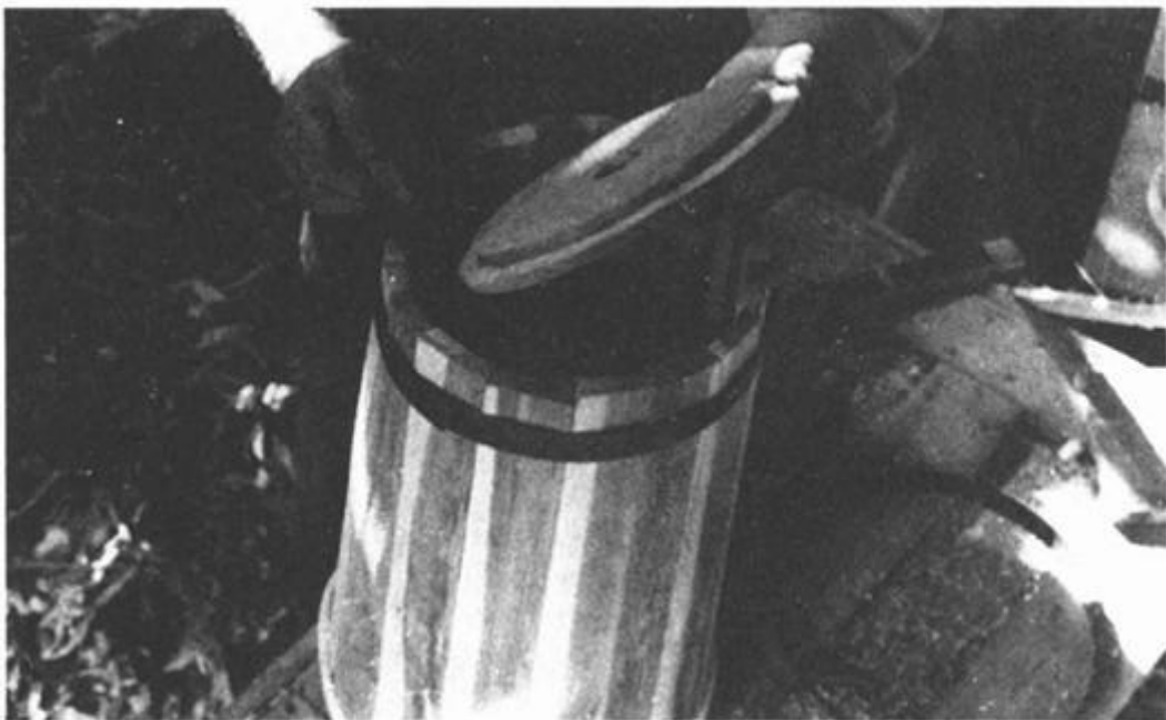
ILLUSTRATION 58 Step 23: For the lid, obtain the circumference using the same procedure as for the head ( ILLUSTRATION 27 – ILLUSTRATION 36 ). For groove on
