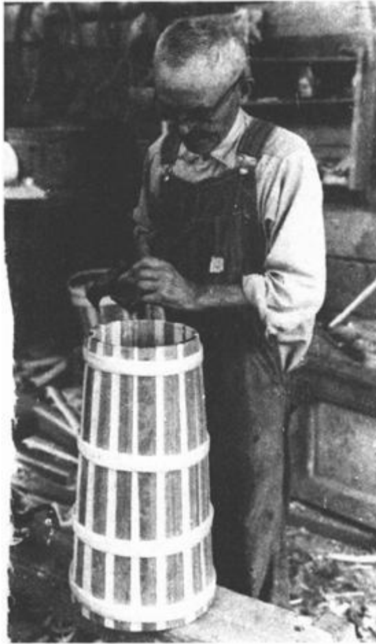
ILLUSTRATION 57 Step 22: Add three more hoops, using the same procedure. With a handsaw, cut off the staves at top to even them. Use a rasp to smooth the top and bevel the edge.
