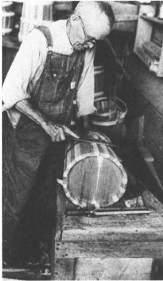
ILLUSTRATION 41 Step 14: With the temporary bands still on, smooth outside of the churn with a wood rasp.
