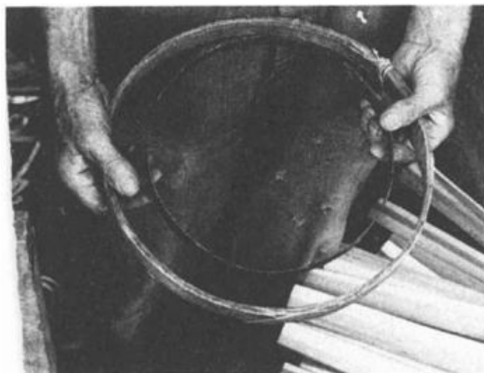
ILLUSTRATION 13 Alex checks his stave angle on the gauge. The correct angle should be maintained as closely as possible for the full length of the stave. However, the angle does not have to be perfect. The wood, being pliable, seats itself. The last stave to be fitted ( Step 5, ILLUSTRATION 18 ) has to be driven into place. This closes most of the cracks which may result from slight errors in the angles of the other staves.
