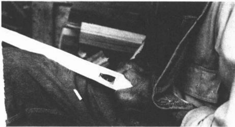
ILLUSTRATION 49 Using a pocketknife, begin to cut out and shape the notch. Continue to shape the notch as shown.
