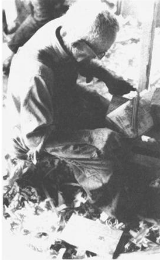
ILLUSTRATION 30 Step 11: Use a shaving horse and drawing knife to smooth both pieces.
