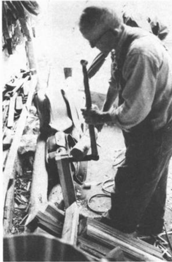
ILLUSTRATION 5 Step 1: Cut the cedar in the fall when the sap is down. Stack it up to dry for about six months. When you're ready to make a churn, split the cedar into staves with a stave froe.
