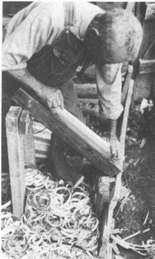
ILLUSTRATION 11 Using a long-jointer, wood is planed from the edges of each stave until the angled edges fit the gauge.
