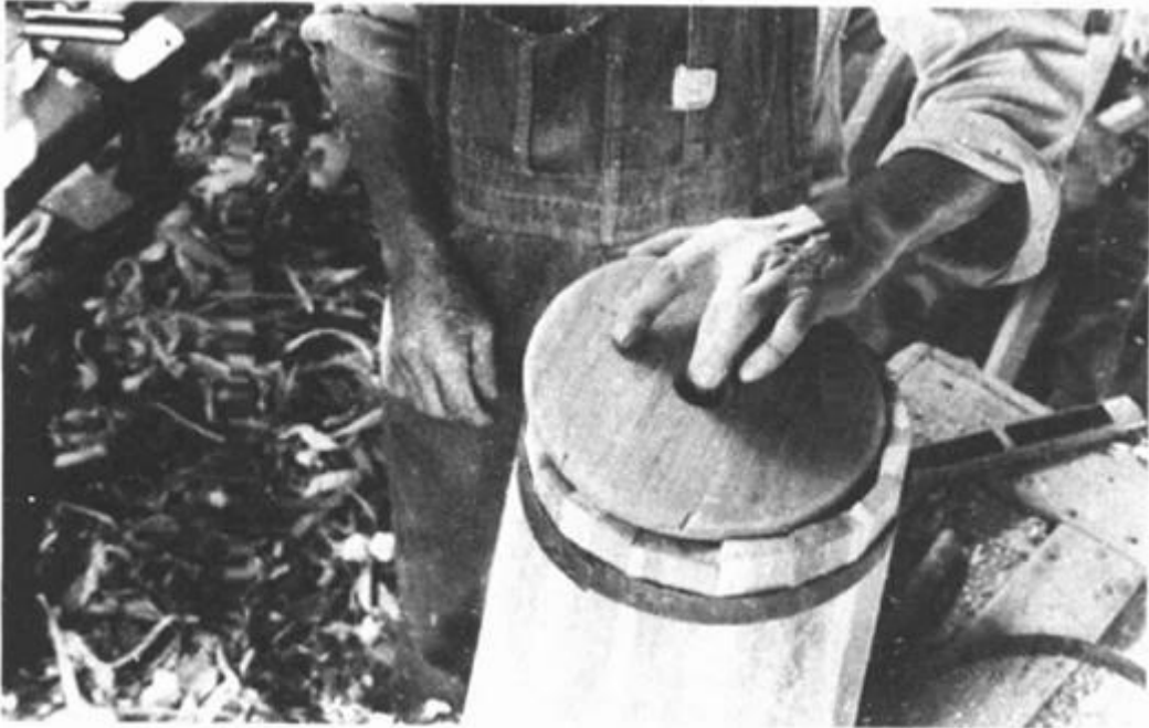
ILLUSTRATION 59 The top should fit right on top of the churn, with a hole in the middle that the dasher handle can easily slide through.
