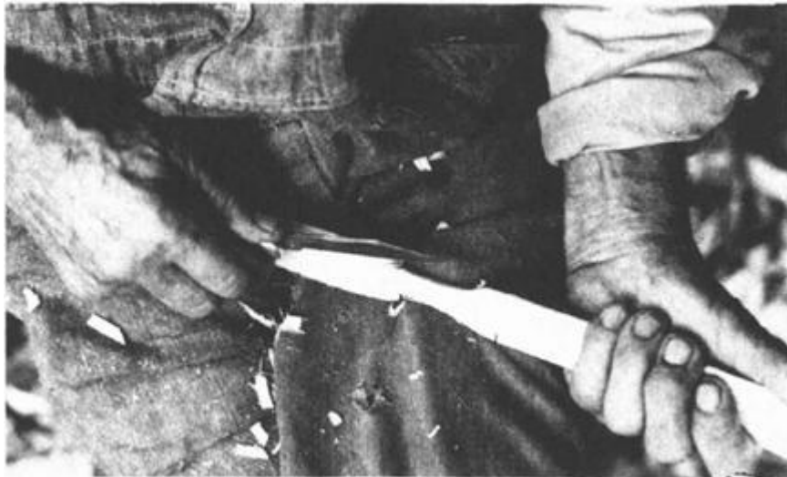
ILLUSTRATION 50 On the opposite end of the hoop, cut with a knife as shown, until the inner side ( ILLUSTRATION 51 ) and the outer side ( ILLUSTRATION 52 ) are finished.
