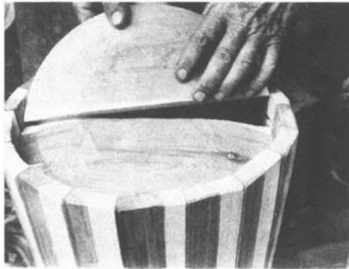
ILLUSTRATION 37 Step 13: Take the bottom (head) hoop off. Fit the two halves of the head into the groove made by the croze. Put another temporary hoop on that fits in the middle of the churn. (Alex replaced the bottom wooden hoop with a metal middle hoop.)
