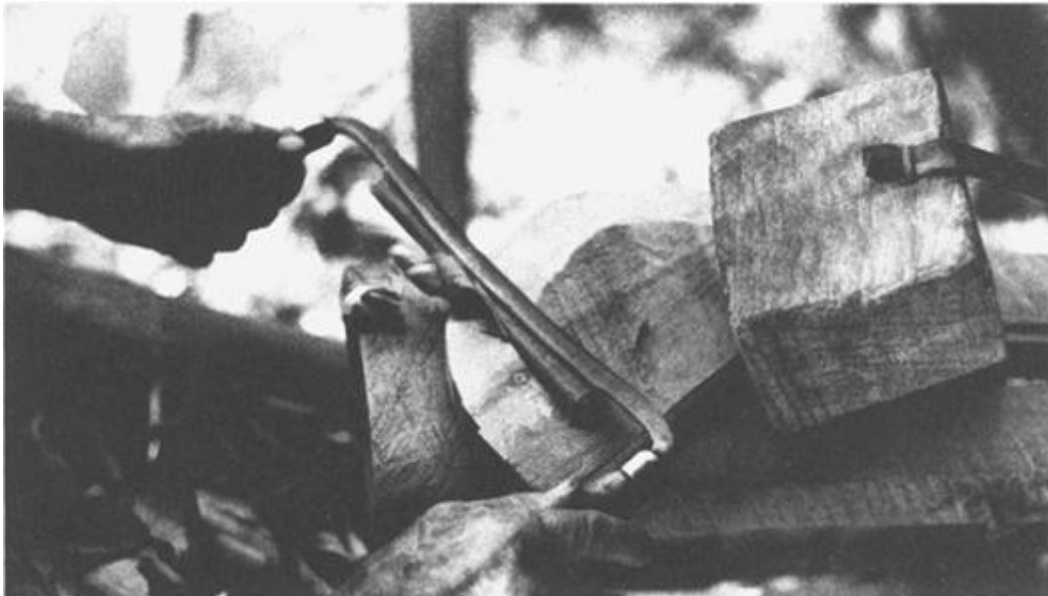
ILLUSTRATION 35 Step 12: Begin to bevel the edges of the half-circles with a drawing knife.
