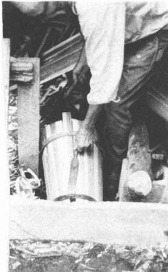
ILLUSTRATION 19 A chisel can be used as shown to help fit the last stave.
