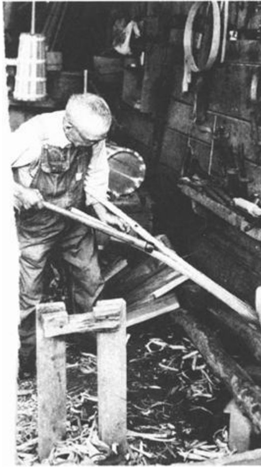
ILLUSTRATION 43 Step 16: For the hoops, use green white oak. If the oak is dry, soak it overnight. Split the oak into strips using a froe and mallet. Measure the length with string, allowing six extra inches for the notch and lock.
