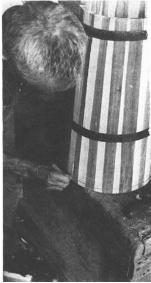
ILLUSTRATION 42 Step 15: To measure for a permanent bottom hoop, take a string and measure the very bottom of the churn.
