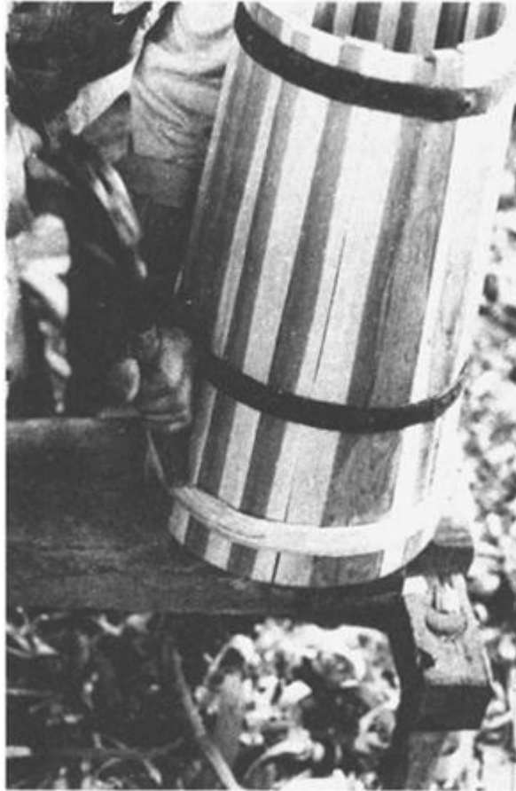
ILLUSTRATION 55 Step 20: Put the hoop around the churn and force it down to the bottom (head) of the churn with a hammer and stick of wood—keep the thick edge of the hoop up, toward the narrow (top) part of the churn.
