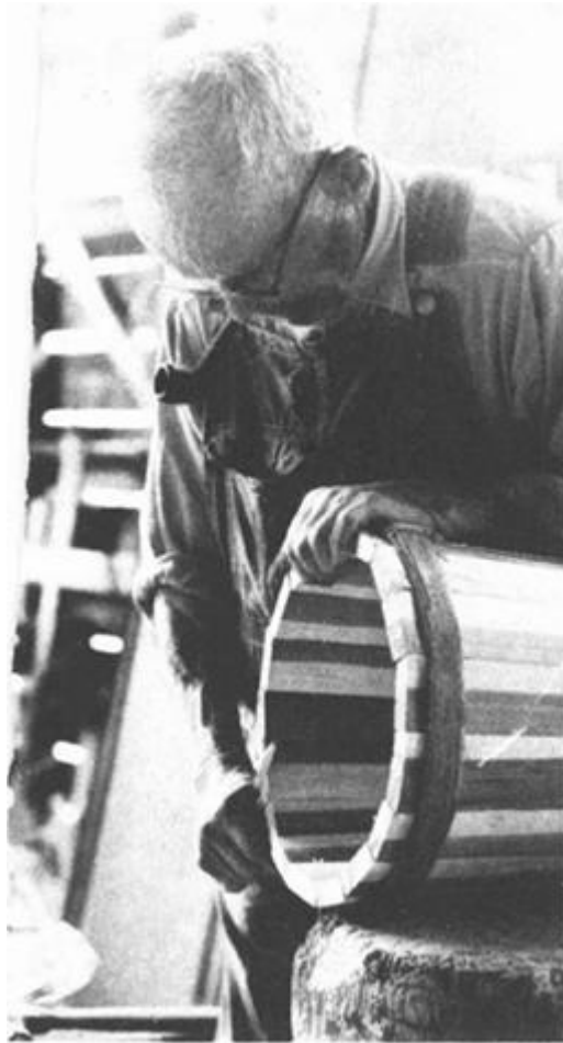
ILLUSTRATION 21 Trim off uneven edges on the bottom with a pocketknife. Use a hammer to adjust the bands to higher or lower positions (for a better fit).
