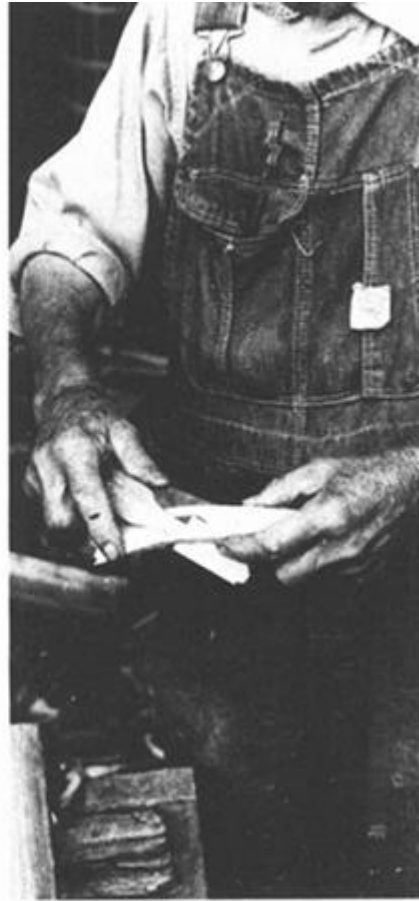
ILLUSTRATION 53 Step 19: Bend the hoop around your knee to make it curve, and hook the ends of the hoop together ( right ).
