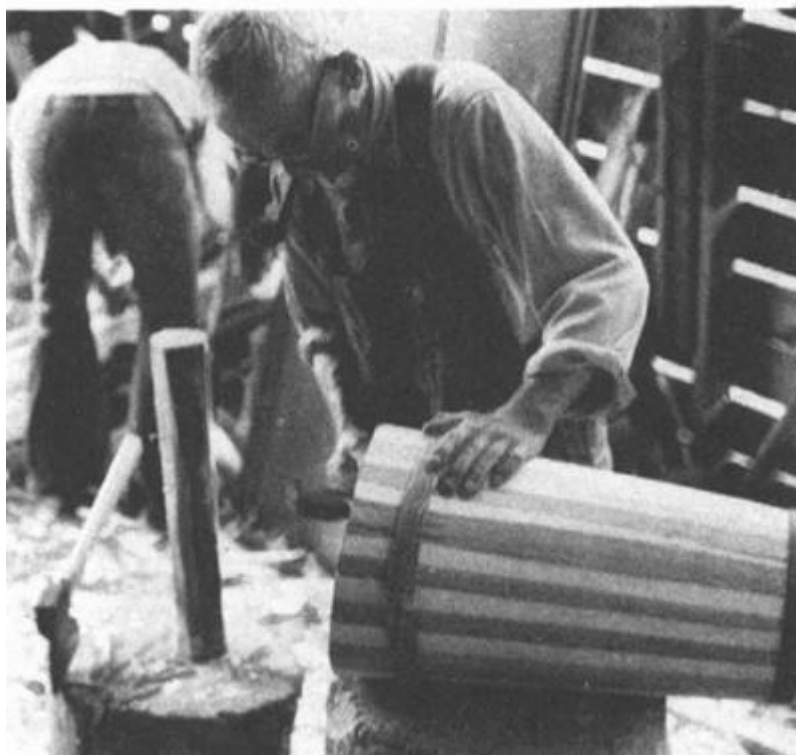
ILLUSTRATION 20 Step 6: Pull out the bag and hammer the staves until they are even.
