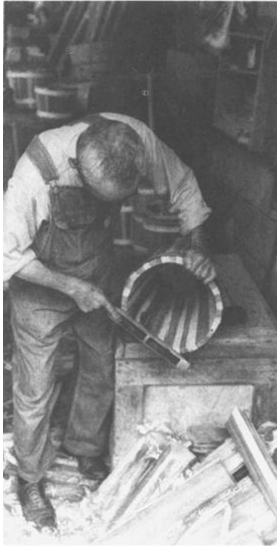
ILLUSTRATION 23 Step 8: Use a rasp to smooth the outer edges of the top and bottom. The churn must sit straight and flat.
