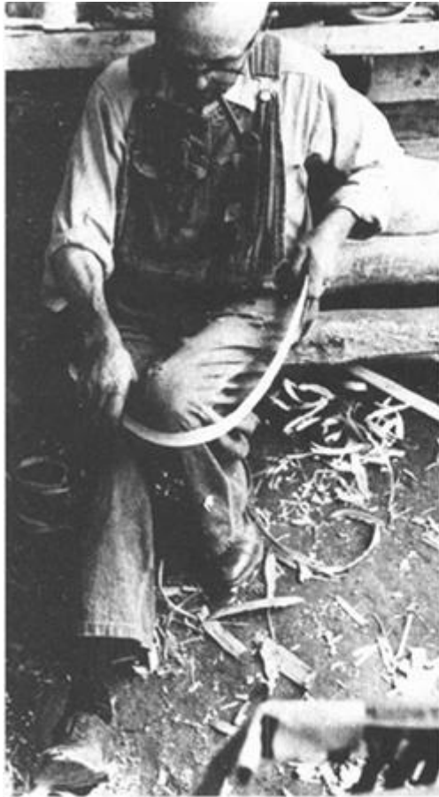
ILLUSTRATION 53 Step 19: Bend the hoop around your knee to make it curve, and hook the ends of the hoop together ( right ).
