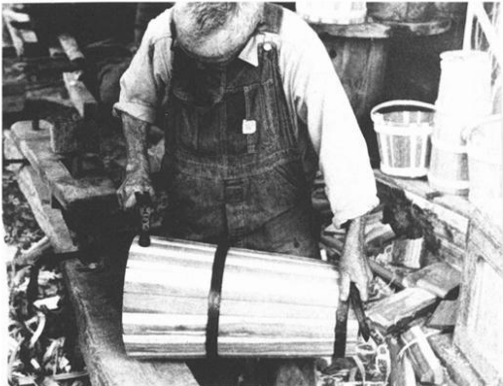
ILLUSTRATION 38 With a chisel and hammer, force the middle hoop down as tightly as possible.
