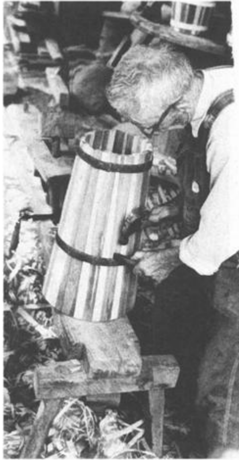
ILLUSTRATION 38 With a chisel and hammer, force the middle hoop down as tightly as possible.
