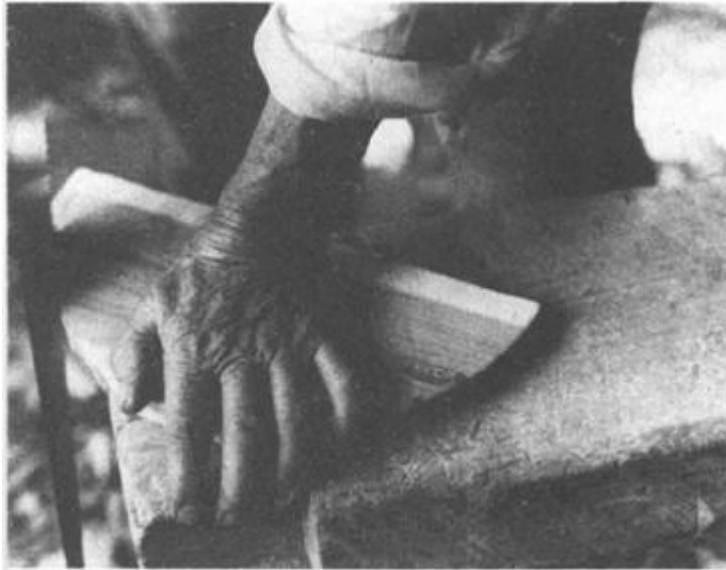
ILLUSTRATION 32 Begin to cut the half-circles out with a handsaw. Saw as close to the edge of the half-circle as possible.
