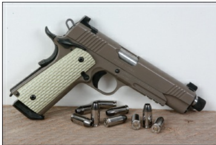
A Kimber full-size 1911 in Desert Warrior mode. The barrel is threaded and the sights are set high for use with a silencer.
