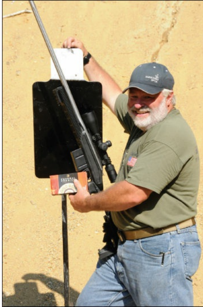
This is a head shot at 1,000 yards. Rifle is a Remington Sendero converted to tactical use. Cartridge .300 Winchester, Federal ammo with 190-grain Sierra bullets.
