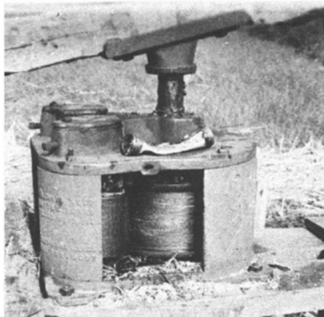
ILLUSTRATION 28 Mr. Brooks's mill has three rollers (one is concealed in this photo).
