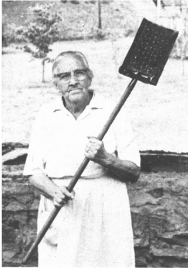
ILLUSTRATION 36 Mrs. Brooks holds the skimmer. Note the holes in its bottom—juice runs through them but foam doesn't.
