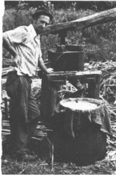
ILLUSTRATION 31 The burlap bag spread over the barrel serves as a strainer. This is the first of three strainings during the entire sorghum-making process.
