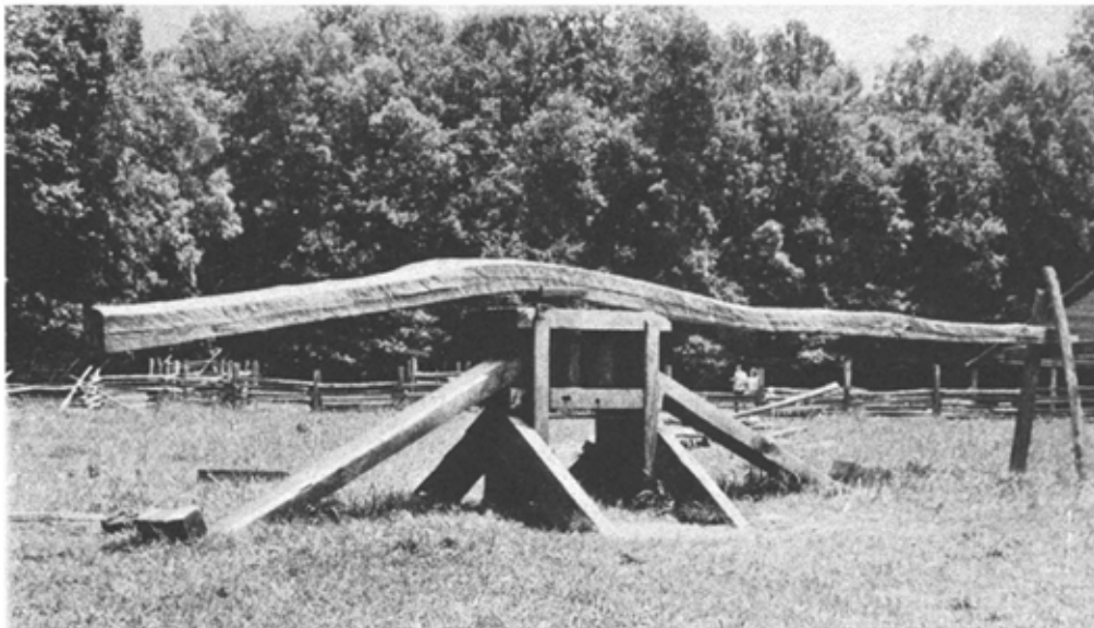
ILLUSTRATION 24 A horse-operated sorghum mill in the reconstructed pioneer settlement at the Cherokee, North Carolina, entrance to the Smokies.
