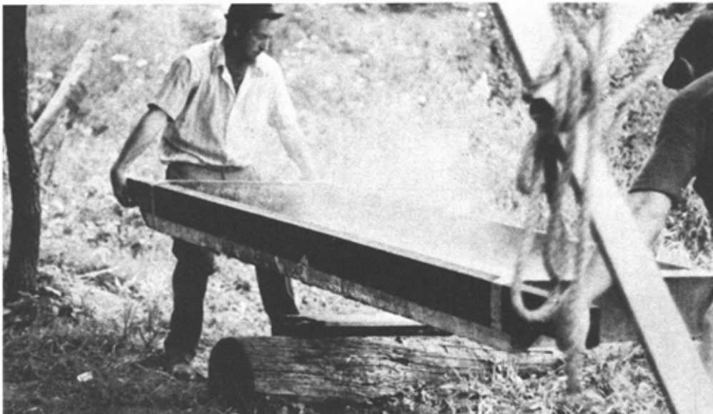
ILLUSTRATION 37 The boiler-box is removed from the furnace.
