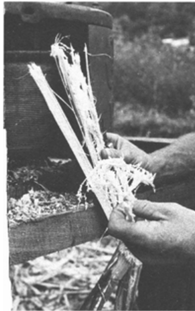
ILLUSTRATION 30 The mill pulverizes the cane, leaving it dry and flaky on the inside. The pulpy ground cane will be spread on fields as mulch. The extracted juice runs into a burlap-covered barrel.
