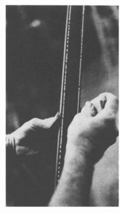
Be very careful from now on, as you are building an instrument you want to be proud of. Keep everything clean; work on a soft rag. A bad scratch or a mistake is hard to overcome at this stage. Remove all excess glue now, or at least mark around a glue spot for removal later. If the glue is not removed, it will make a light or white spot in the finish.
