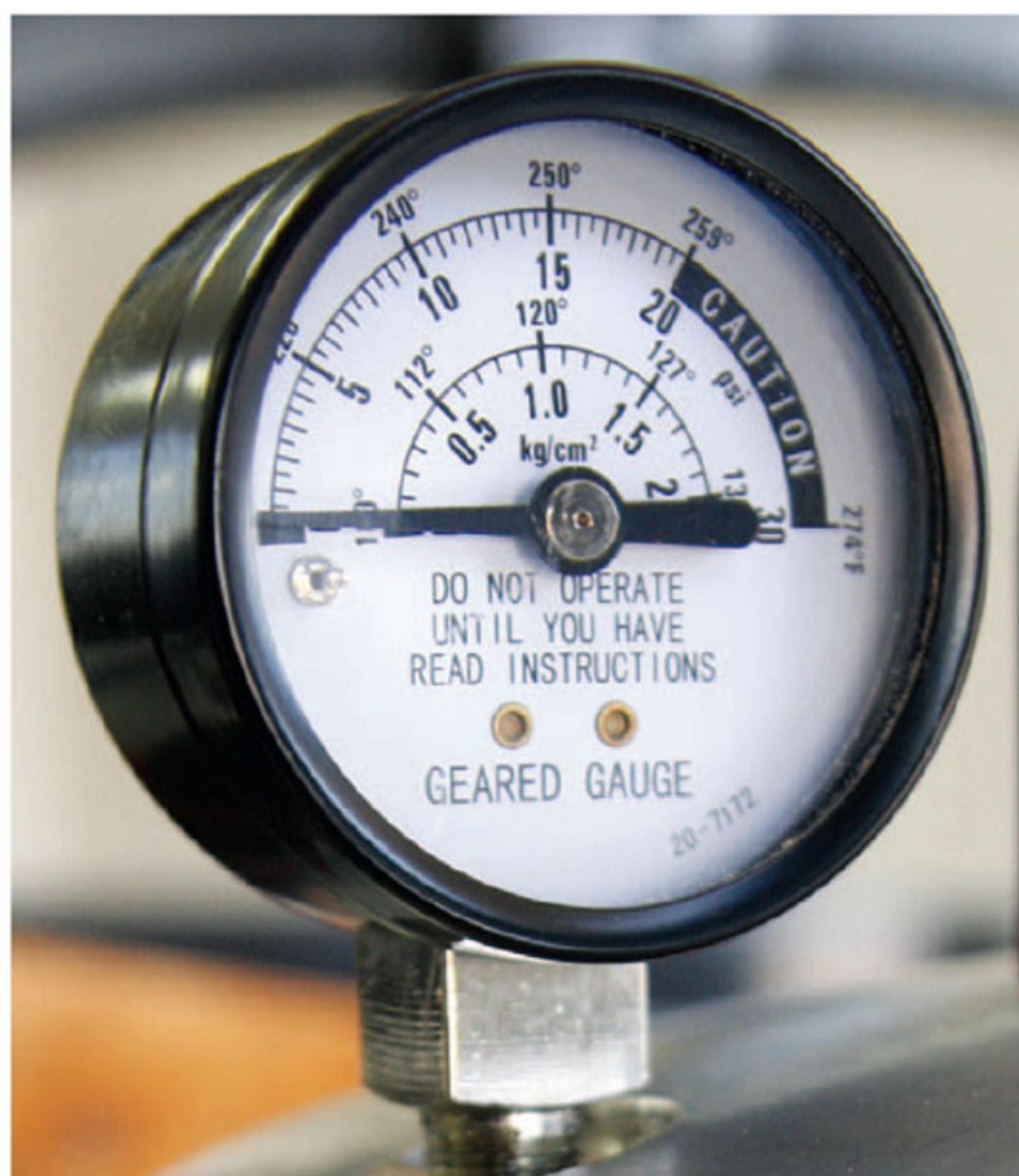
Left: Get dial gauges checked annually. Right: A 21.5-quart canner will process 19 stacked pints.
