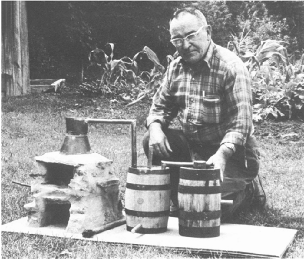
ILLUSTRATION 3 Buck Carver kneels behind a one-gallon still he made for the Foxfire museum. The still is authentic in every detail from the flue of the furnace to the tin-locked copper joints in the cooker and condenser to the chestnut barrels Bill Lamb made for the model.
