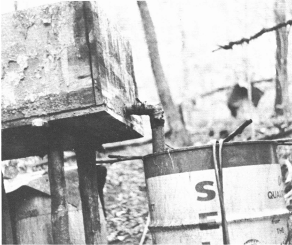
ILLUSTRATION 16 The heater box from the other side, showing the connection between the heater box and the condenser which is mounted in the metal drum.
