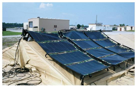
Three CIGS arrays of four panels, each suspended by rope or cable demonstrate their flexibility.
