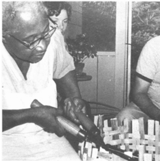
ILLUSTRATION 20 At the top, the ends of the ribs will probably be uneven. Before the rim can be made, these must be trimmed off straight. This can be done with a knife or, as shown here, with a pair of hedge clippers.
