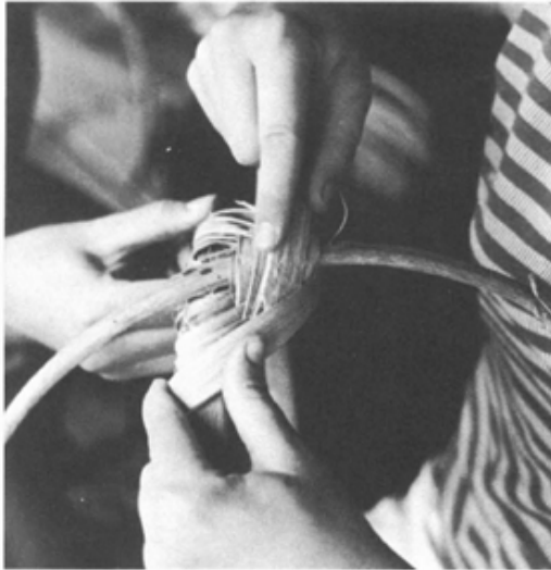
ILLUSTRATION 26 When one split runs out, tuck in its end, insert the point of another into the weave, and continue ( left ). When the weaving is progressing well at both hoop intersection points, insert the first two ribs. Simply force their sharpened ends into the weave ( right ).
