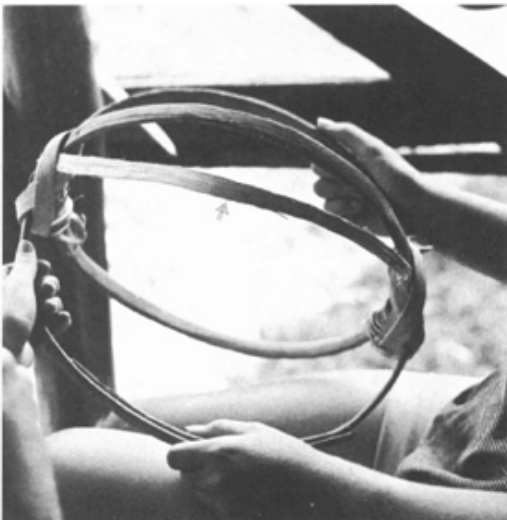
ILLUSTRATION 27 The first rib in place (arrow) ( left ). Continue weaving as before ( right ) ...
