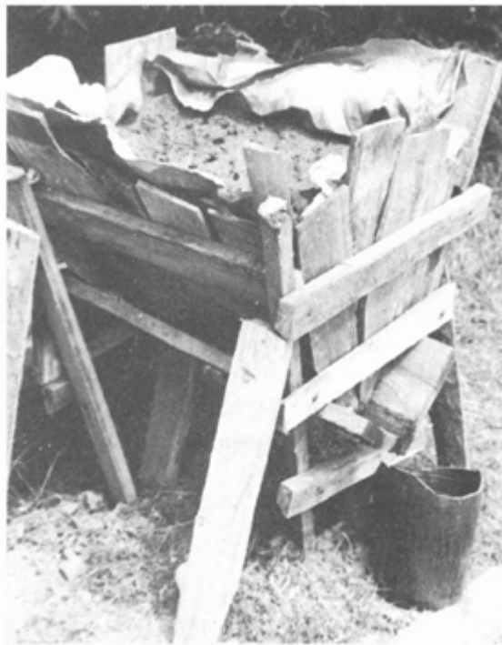
ILLUSTRATION 6 A crude ash hopper, lined with paper and filled with hickory ashes, stands ready to work.
