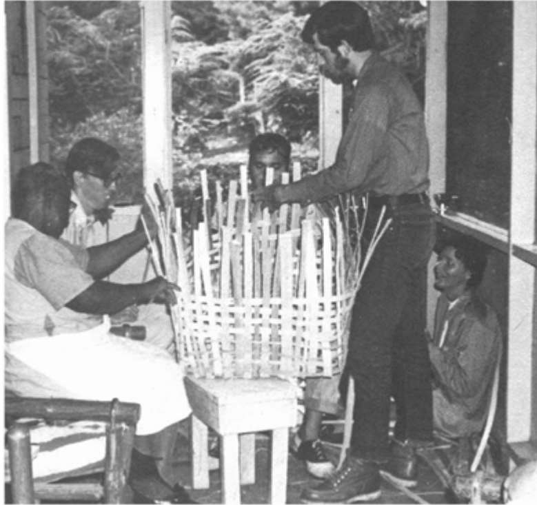
ILLUSTRATION 19 Continue weaving until the top is reached. This will take nearly all the splits you can make from two good oak saplings. When the end of one split is reached, simply lap a new one over the end of the old by about two inches and continue as before.
