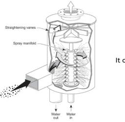
Wet Scrubbers: air pollution control devices for removing particles and/or gases from industrial exhaust stream
