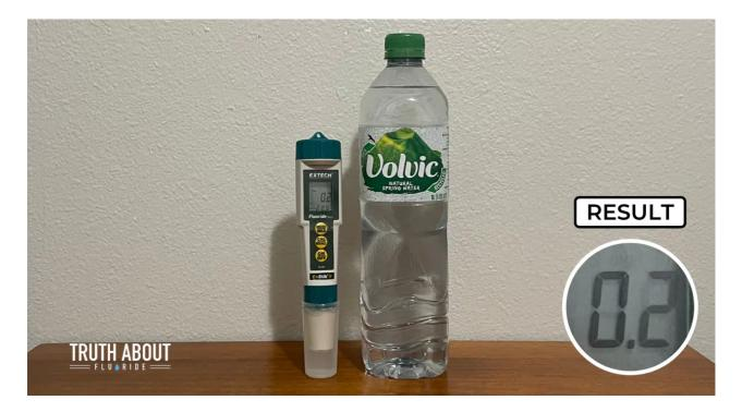
According to the fluoride meter, Volvic natural spring water contains 0.2 ppm of fluoride.
