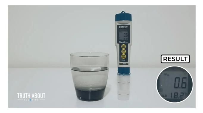
According to the fluoride meter, there is 0.6 ppm of fluoride in the water <u>before</u> filtering.
