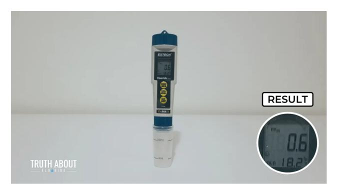
The fluoride meter detected <u>0.6 ppm</u> of fluoride in the tap water.
