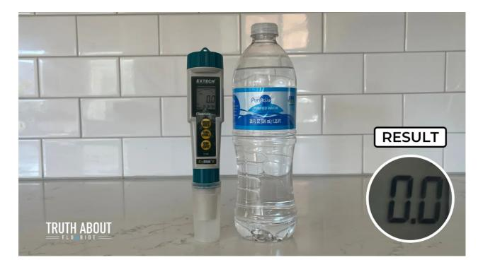
According to the fluoride meter, Aldi's PurAqua purified water and Italian mineral water are fluoride-free as the test results showed both bottles contain 0.0 ppm of fluoride.
