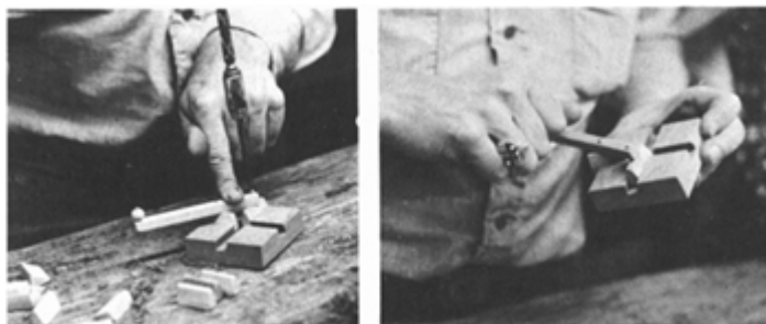
ILLUSTRATION 11 Dave puts wax on the pistons to reduce friction and keep them from binding, then he screws a bead into the handle for ease in turning. Last, he sets the two pistons into the channels cut in the block and attaches the handle. The screws are left loose so the pistons and arm turn
