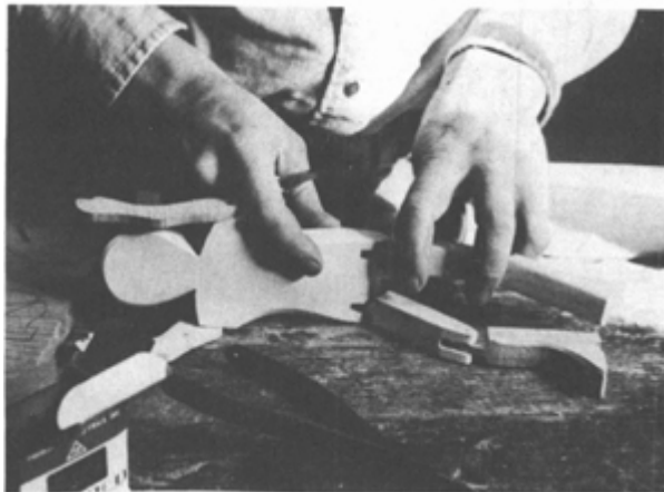
ILLUSTRATION 71 Dave checks to make sure the thigh fits and will swing freely.
