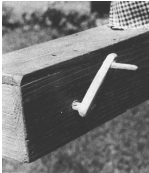
ILLUSTRATION 17 The wooden crank, carved with a pocket knife.
