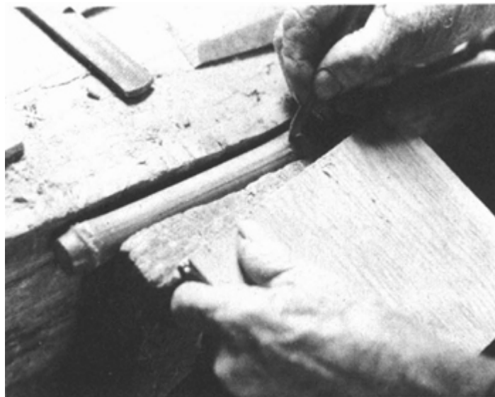
ILLUSTRATION 26 Next he decides which section to use for the “stringed” portion, and, with a pencil, outlines the areas to be cut away.
