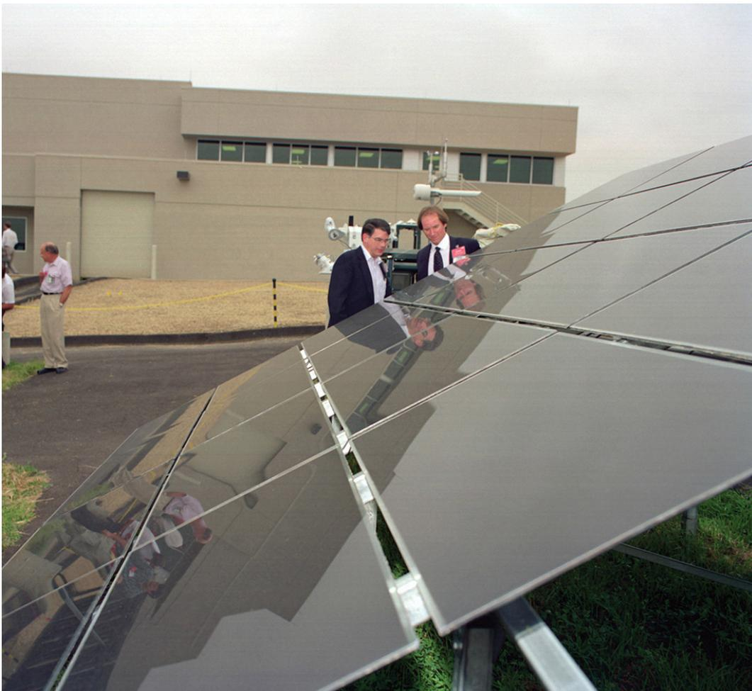
*A ground-mounted cadmium tellurium PV solar array used for research. Cadmium tellurium is often referred to as “CdTe.”*
